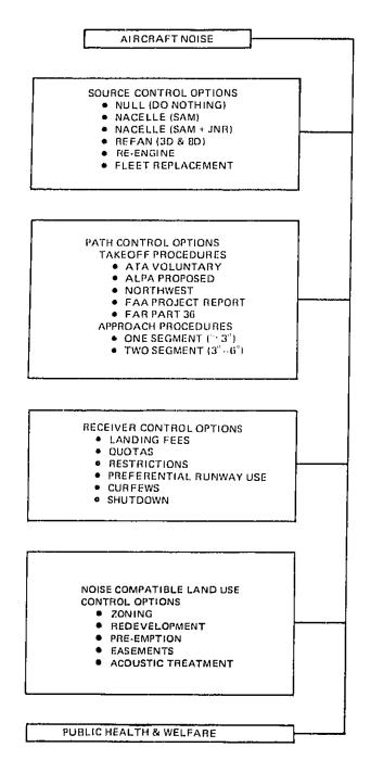
Figure 2-1. Typical Aircraft Noise Control Options.
