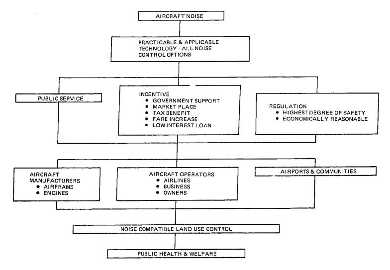
Figure 2-4. Exploitation of Source Control Options.
