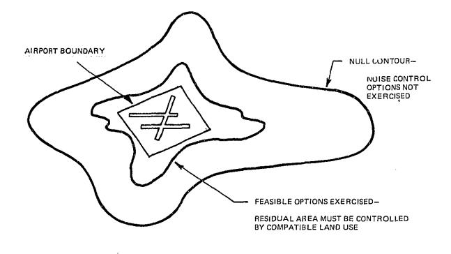
Figure 2-5. Noise Exposure Contours for Levels Representing Various Options
